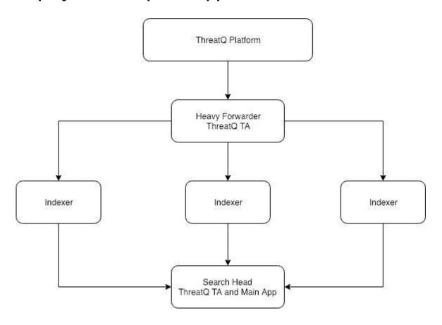
For a distributed environment with a **cluster of search heads**, you will need to configure the ThreatQuotient Add-on App on the master node and use the Splunk App deployer to propagate that configuration to all nodes.
