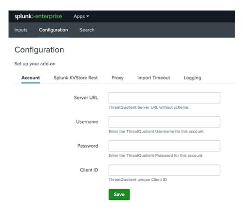
Upon clicking the **Save** button, you can see the status of the Authentication action. If the ThreatQuotient appliance is down, and/or the authentication parameters are invalid, an error message will be displayed. Unless the appliance is up and the authentication parameters are valid, this App will not work.
